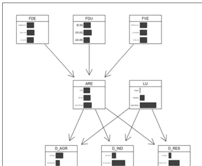
Figure 10.3 CONF_2 - BN model for multi-sectoral flooding damages assessment with associated variable marginal distributions
