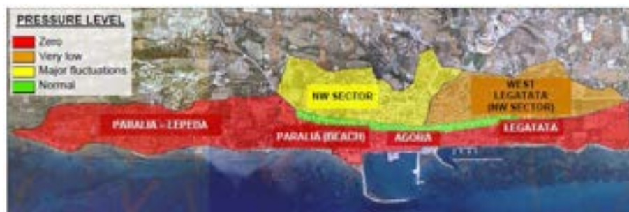
Figure 5.7 Rapid network assessment in Lixouri after the second earthquake. Source: EYDAP 2014
